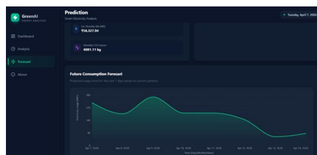
Fig. 6. GreenAI Forecast Tab (Industrial Dataset): Est. monthly bill Rs. 58,327.94 and CO 2 impact 6,081.11 kg. Seven-day projection shows declining trend to ~90 kWh.
